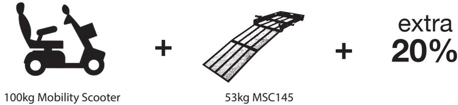
$$\begin{aligned} & \text{(mobility device + Carrier)} && 100\text{kg} + 53\text{kg} \\ & \text{(Adding extra 20\%)} && 153\text{kg} + 20\% \\ & && = 183.6\text{kg} \end{aligned}$$
